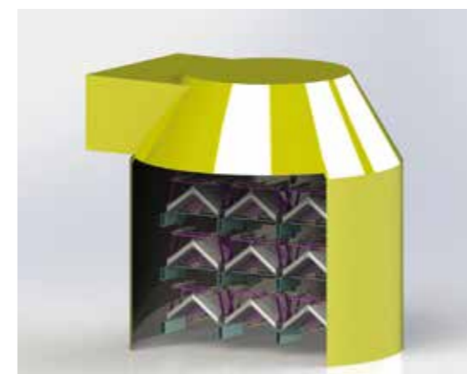
Three-stage roof design mist eliminator plus one-stage tubular design combination with six level water wash pipe system
