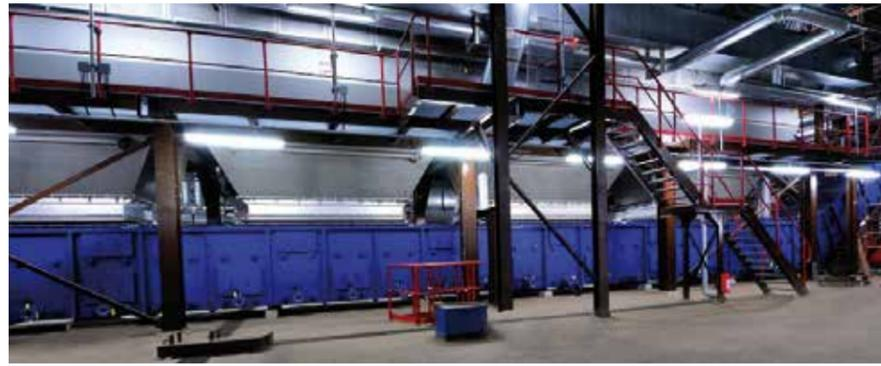
transferred to the head of the conveyor together with the freshly accumulated bottom ash. The tension of the two steel chains is kept constant by an automatic hydraulic tensioning device. The system is equipped with end switches and scales to monitor the take-up path during operation. Sensors for remote monitoring of the chain tension and the oil temperature are also provided.
