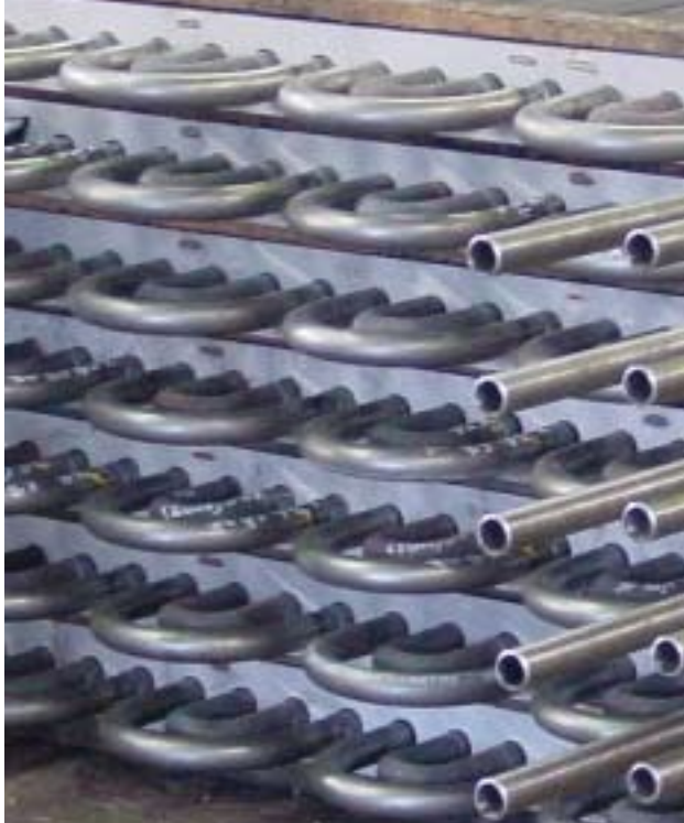
Helical finned tube after 4,000 hours operation
