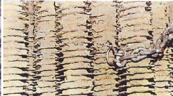
Helical finned tube after 4,000 hours operation
